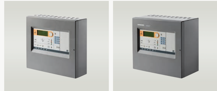
Fire control panel (1L, Compact) FC361-ZZ – Housing: 402x372x132 mm – Batteries: max. 2x 12 V, 12 Ah Order no.: S54433-C112-A1 Fire control panel (1L, Comfort) FC361-ZA – Housing: 402x372x211 mm – Batteries: max. 2x 12 V, 25 Ah Order no.: S54433-C111-A1
