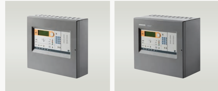
Fire control panel (2L, Compact) FC362-ZZ – Housing: 402x372x132 mm – Batteries: max. 2x 12 V, 12 Ah Order no.: S54433-C119-A1 Fire control panel (2L, Comfort) FC362-ZA – Housing: 402x372x211 mm – Batteries: max. 2x 12 V, 25 Ah Order no.: S54433-C120-A1
