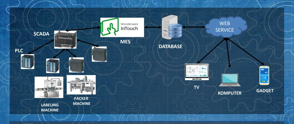
Machine -> MES PLC -> SCADA -> Database -> Web Service -> Desktop/Laptop/Gadget
