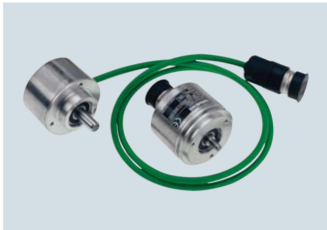
Incremental encoder (sin/cos 1 V_{pp} /RS422/HTL) with cable and connector, clamp flange or Synchro flange
