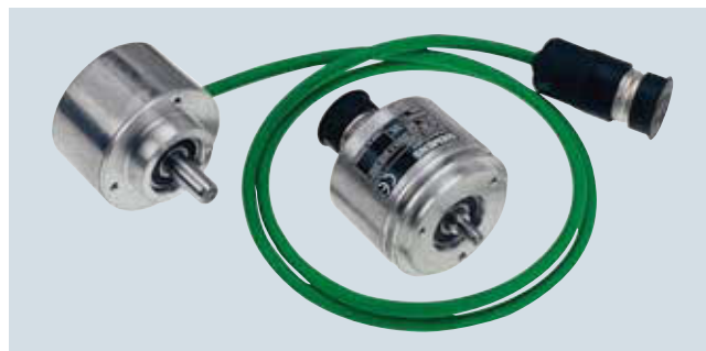
Incremental encoder with sin/cos 1 V_{pp} and clamp flange incl. cable with connector as well as incremental encoder with RS422 and Synchro flange
