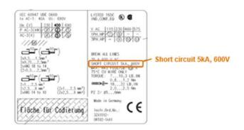
Example: name plate Siemens contactor
