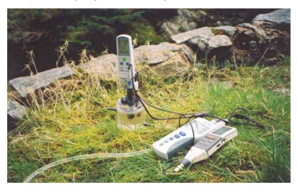
Figure 4.1 Measuring pH, Eh and DO in a flow-through cell.
