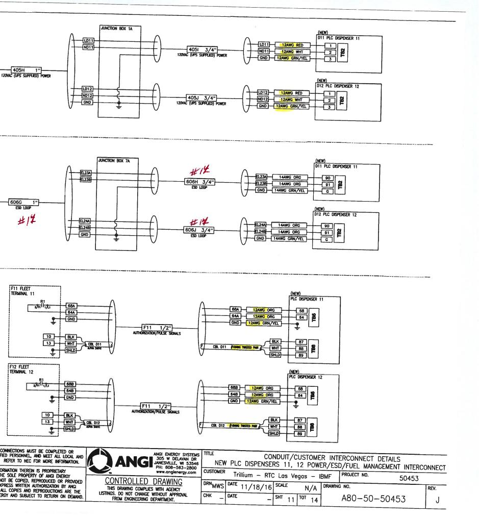
ALLOW FOR 10% SPARE CONDUCTORS IN ALL CONDUITS
