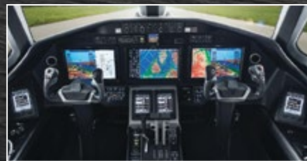
Citation Longitude features the next evolution of the Garmin™ G5000™ flight deck, with three large 14" glass displays, four touch-screen controllers and fully integrated autothrottles.
