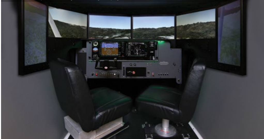
Redbird’s FMX is an enclosed simulator with multi-screen visuals and software that can mimic dozens of aircraft. It fits in a 16’x16’ space with an eight-foot ceiling, and plugs into a normal wall outlet. Redbird Photo
