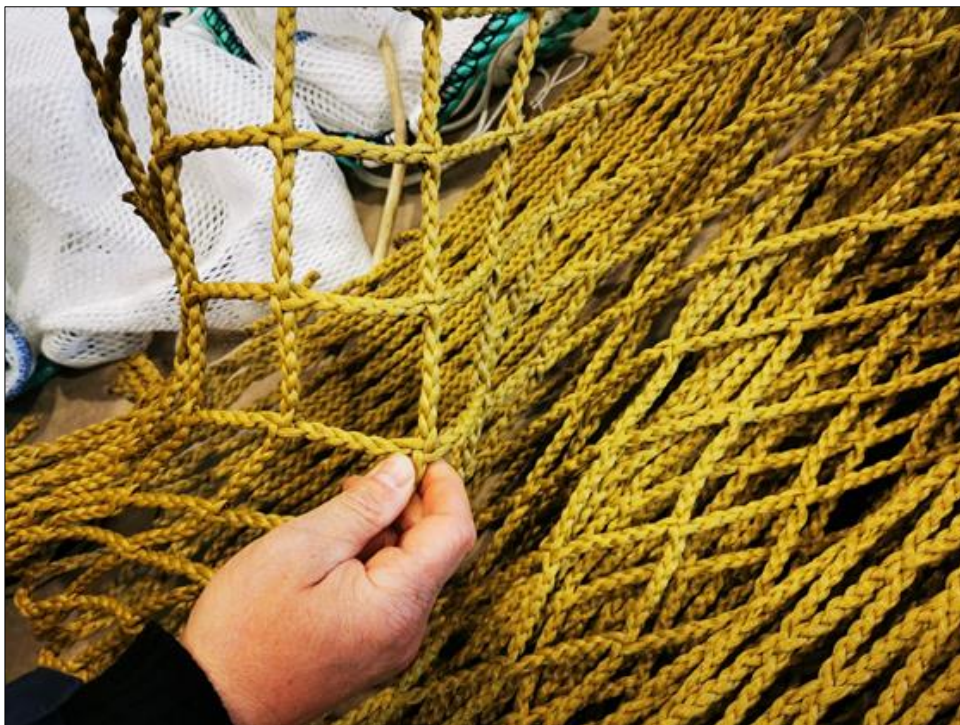
Image 2-4. Top: Retention System netting (10 × 10 mm); Bottom: Retention Zone entrance bottom netting with increased mesh size (50 × 50 mm).
