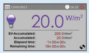
ClimaPlus controller specific for Photostability chambers with automatic integration of VIS and UV sensors and light meters according to traceability standards. Enables automatic running (with auto-stop) of test programs and FDA 21 CFR compliant data logging.
