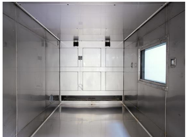
Interior view of FitoClima 8.000 with lateral observation window
