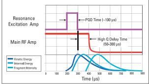
Figure 1: Schematic of dissociation process
