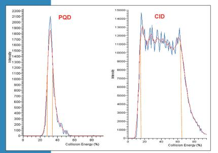
Figure 3: Collision-energy optimization for both PQD and CID using peptide F\*ESNFNTQATNR from lysozyme (\*Indicates TMT<sup>6</sup> label)
