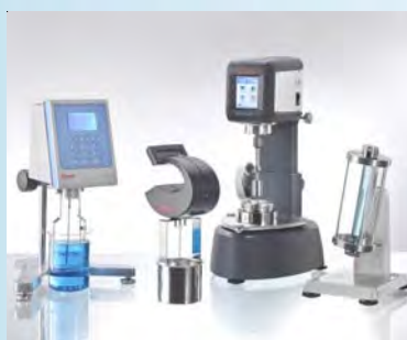
Selection of falling ball and rotational viscometers for fast, reliable viscosity measurement for raw material evaluation or batch testing
