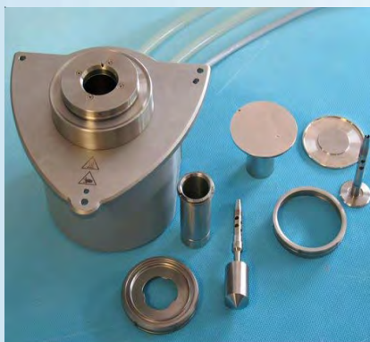
Peltier temperature module for cylinders (TM-PE-C) with adapter for use with plate and cone measuring geometries as well as selection of plate and cylinder geometries
