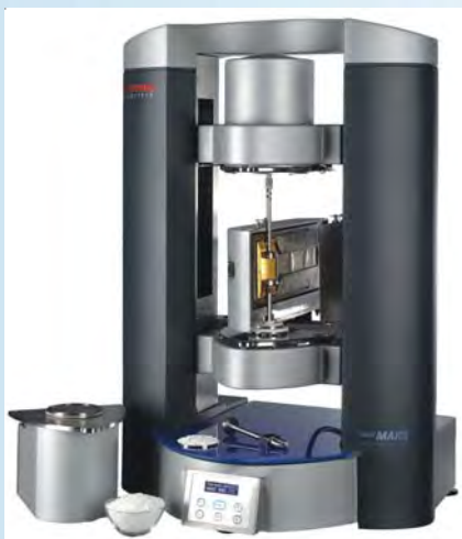
HAAKE MARS with CTC and clamps for measuring solids, SER tool for extensional rheological measurements and RheoScope unit
