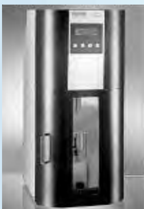
Mini-injection molding machine with various molds for the production of specimens for rheological tests: disk-shaped, in various diameters, for plate/plate measuring geometries or rectangular for the solid clamp
