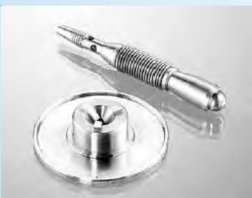
Measuring cells for determining the tribological behavior of material combinations with or without lubricants
