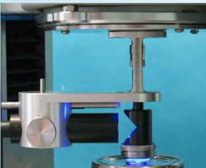
Measuring cell for thermal assisted UV curing
