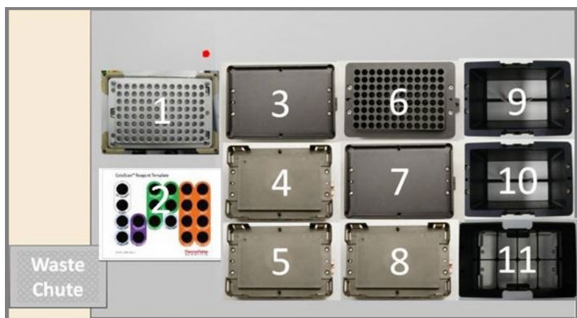
Figure 3 CytoScan™ deck configuration for the NIMBUS™ Instrument.
