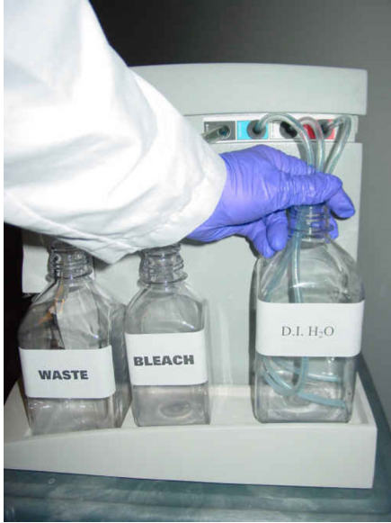
Figure 41 Cleaning the wash and water lines.
