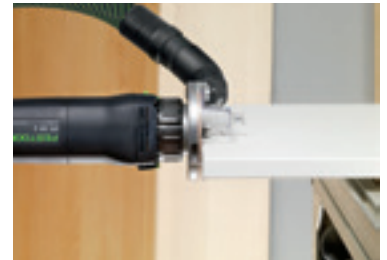
Rounding plastic or solid wood veneer.
