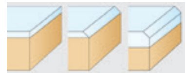
Flush Chamfered Flush + chamfered
