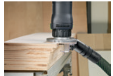
Chamfering plastic or solid wood veneer.
