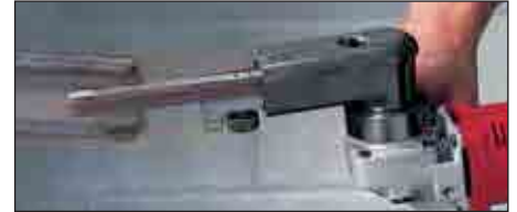
Grind and deburr ends of metal stock.
