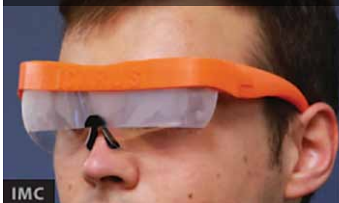
ICARUS uses polymer dispersed liquid crystal technology to create a view-limiting flight training device with the flick of a switch. Photos courtesy of Nick Sinopoli
