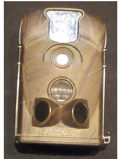
This “LTL Acorn” scouting camera is a regularly used device to monitor animals in captivity and in the wild. It takes videos or motion sensed photos. Photo J.Marten
