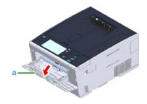
Slightly lifting the MP tray (a), press the right arm (b) inward, then unlock the tab (c).
