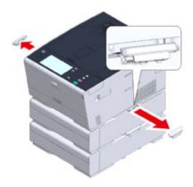
Lift up the machine to remove the additional tray unit.
