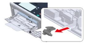
Remove the fusing unit from the machine. For details, see "Replacing the Fuser Unit". Attach the envelope lever to the fuser unit.
