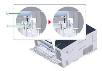
Closing the MP tray without putting the tab back in place may crack the paper set cover. Be sure to put it back in place.
