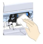
Keep pressing the center of the MP tray, wipe the separation roller (e) with a wet cloth that has been wrung out well.
