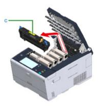
Hold the handle of a new fuser unit, align the fuser unit to the grooves behind the toner cartridges, place the fuser unit into the machine.
