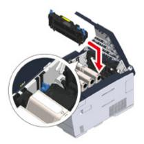
Tilt back the fuser unit lock levers (b) to lock.
