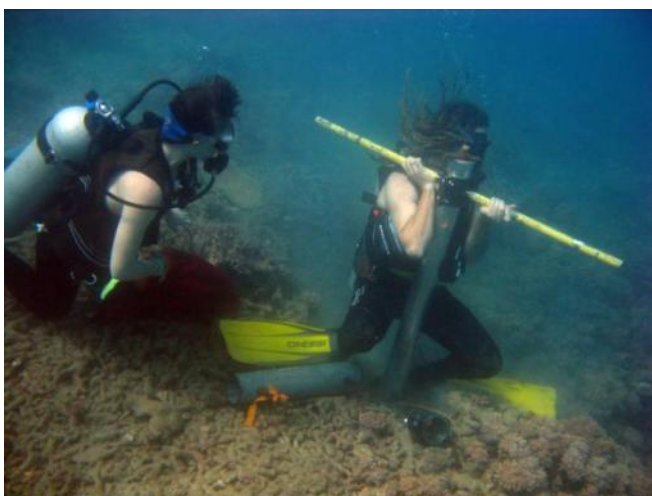
Coring through dead Acroporid reefs in the Palm Islands
