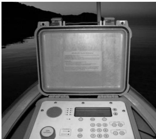
Fig.1: (a) Individuals of Siganus lineatus are tagged by inserting an acoustic transmitter (Vemco, V9-1L, 9mm x 24 mm) into the peritoneal cavity, released back onto the reef and then (b) tracked over continuous 24 hour periods from a kayak equipped with (c) an acoustic hydrophone (Vemco, VH110) and (d) receiver (Vemco, VR100). Photos: J Donelson
