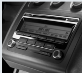
RCD 310 radio / CD player DAB-enabled sound with four speakers (standard fit with satellite navigation)
