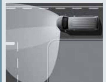
Fog lights with cornering Reduce the risk of accidents by lighting up the road in the direction you're turning
