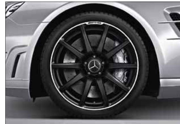
AMG 10-spoke forged wheels painted matt black and with a high-sheen rim flange, with 255/35 R 19 front tyres and 285/30 R 20 rear tyres (option, only for AMG models, Code 767).
