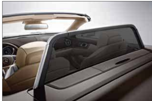
The electric draught-stop minimises draughts in the interior of the open vehicle.
