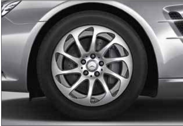
10-spoke light-alloy wheels, painted titanium silver, with 255/45 R 17 tyres (standard for SL 400, Code 25R).
