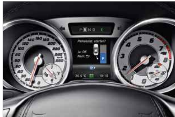
Active Parking Assist shows the driver suitable parking spaces and can carry out the parking manoeuvre if required.
