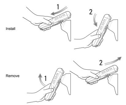
Figure 8-4 Hooking the MC9500-K onto a Four Slot Cradle
