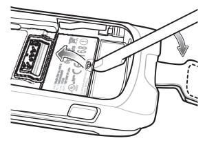
Figure 1-8 SIM Card Cover Removal
