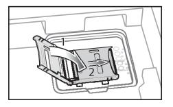
Figure 1-7 Insert microSD Card in Holder
