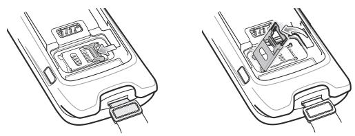
Figure 1-9 Lifting the SIM Cover
