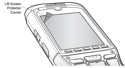
Figure 9-1 Removing the Screen Protector
