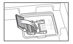
Figure 1-4 Insert microSD Card in Holder
