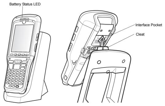
Figure 8-2 MC9500-K Battery Charging
