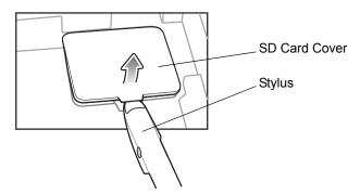
Figure 1-5 SD Card Cover Removal
