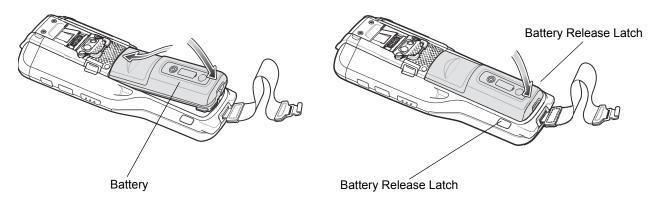
Figure 1-11 Inserting the Battery
