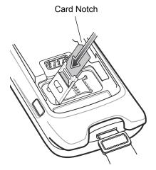
Figure 1-10 Inserting the SIM Card
