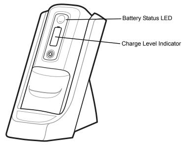
Figure 2-7 Spare Battery in Single Slot Battery Charger
