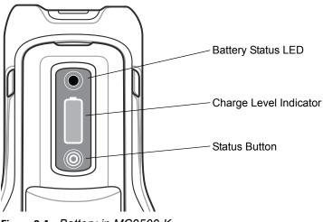
Figure 2-4 Battery in MC9500-K
