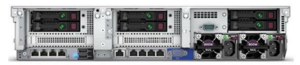
Figure 2-51 HPE ProLiant Gen10 rack servers are based on industrystandard x86 architectures
