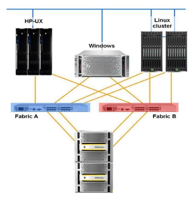
Figure 5-7 A SAN should always be redundant and resilient in design
