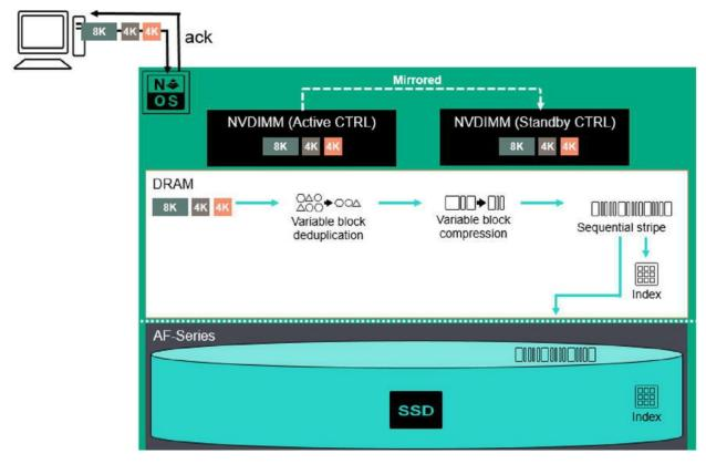
Figure 5-20 Write operation
