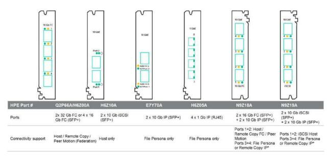
Figure 5-52 A variety of adapters to meet connectivity requirements
