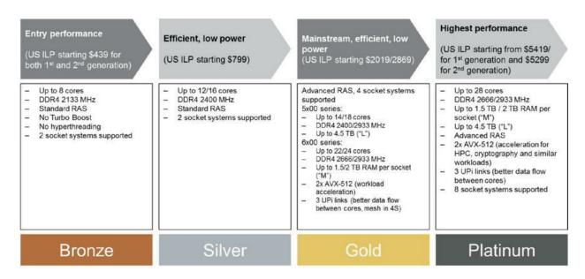
Figure 2-20 Gen1/Gen2 Intel® Xeon® Processor
