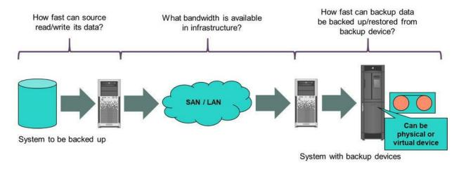
Figure 5-72 Backing up data over the SAN/LAN
