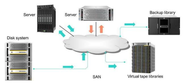
Figure 5-8 Utilizing the SAN for backups and restore operations
