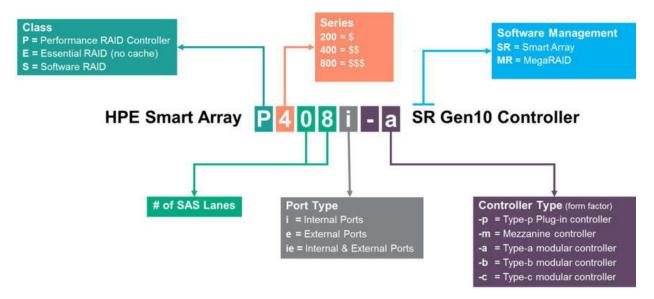
Figure 2-30 Gen10 Smart Array naming framework
