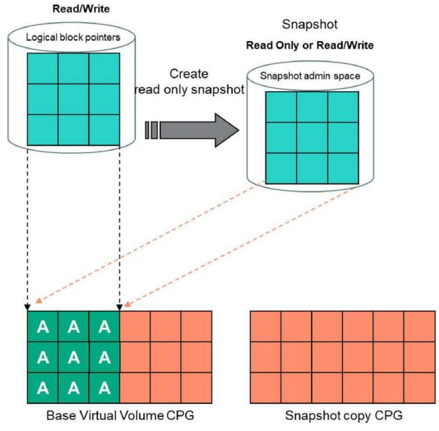
Figure 5-74 The snapshot points to all the original data
