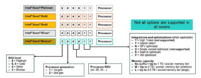
Figure 2-19 Intel<sup>®</sup> Xeon<sup>®</sup> Scalable Family processor numbering and features
