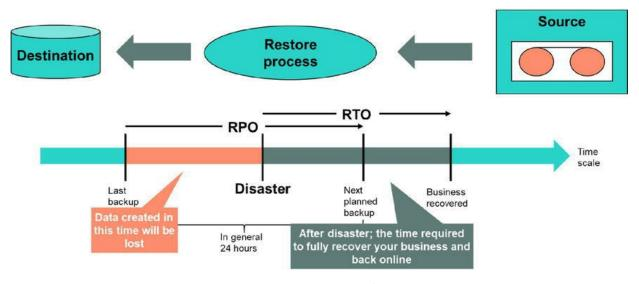
Figure 5-71 Restoring data form a backup
