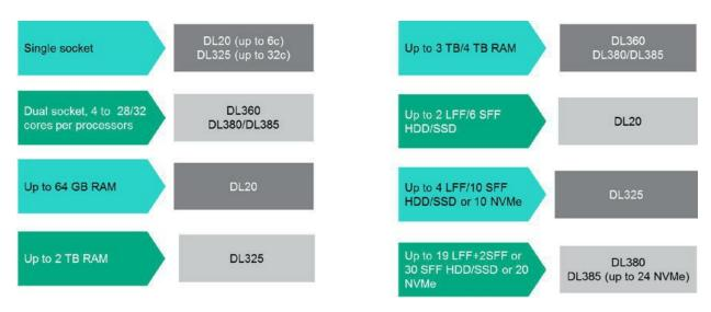
Figure 2-49 Selecting an HPE DL server platform, based on performance, memory, and storage requirements
