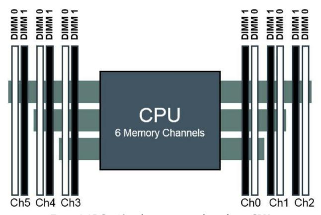
Figure 2-25 Gen10 with six memory channels per CPU
