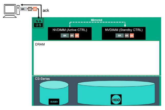
Figure 5-40 HF-Series write operation beginning
