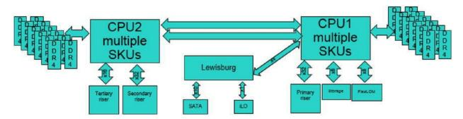
Figure 2-65 ProLiant DL380 Gen10, system/block diagram
