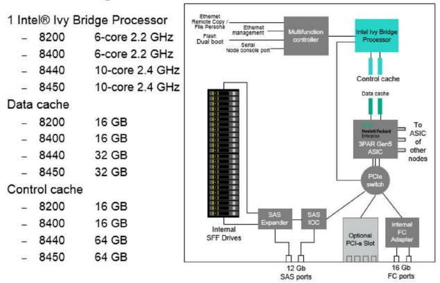
Figure 5-54 The core components of the HPE 3PAR StoreServ controllers
