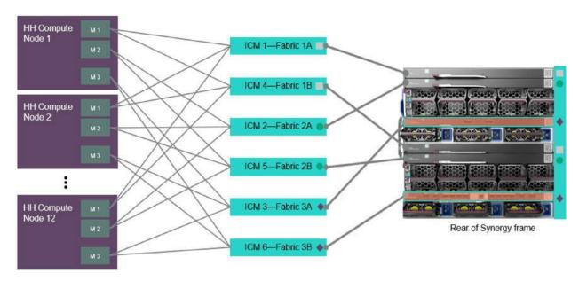
Figure 2-86 HPE Synergy frame interconnect module mapping
