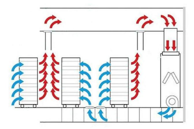
Figure 2-38 Rack placement for proper airflow in a data center with a suspended ceiling and raised floor
