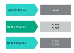
Figure 2-50 Selecting an HPE DL server platform, based on size and expansion requirements
