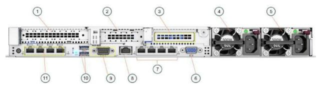
Figure 2-60 ProLiant DL360 Gen10 Server, rear system detail
