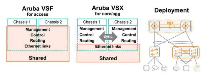
Figure 3-15 Aruba virtualization and HA solutions for access and core
