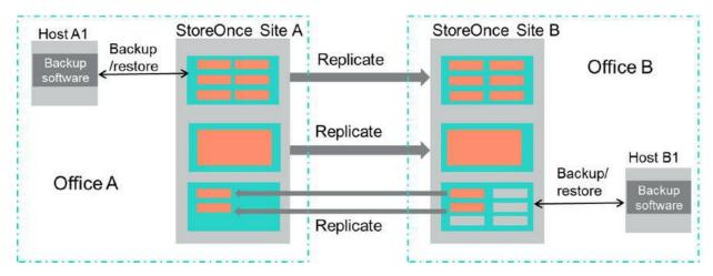
Figure 5-82 Bidirectional replication
