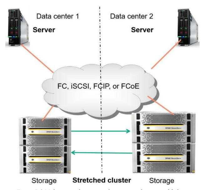
Figure 5-9 Multi-site replication to eliminate single points of failure
