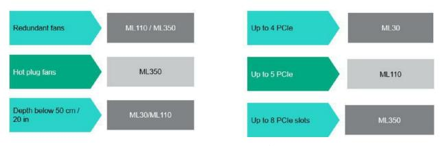
Figure 2-7 Selecting an HPE ML server platform, based availability and expansion requirements
