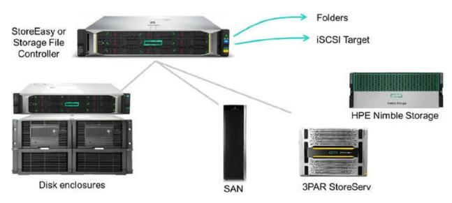
Figure 4-5 Centralized management interface to consolidate storage from DAS, NAS, and SAN
