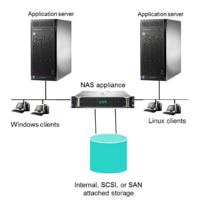
Figure 4-4 Network-attached storage
