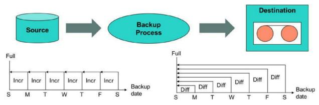
Figure 5-70 Incremental and differential backups
