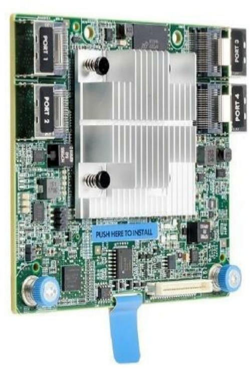
Figure 2-28 HPE Smart Array Controller
