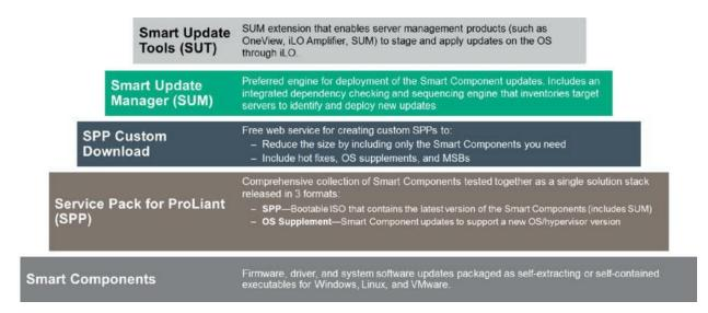
Figure 2-126 HPE Smart Update solution stack
