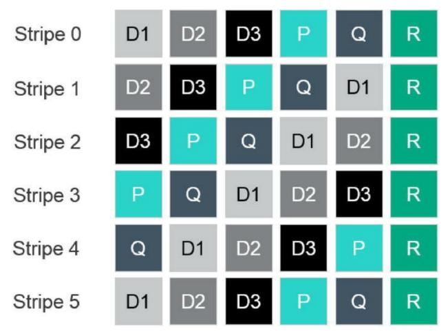
Figure 5-43 HF-Series triple+ parity RAID layout
