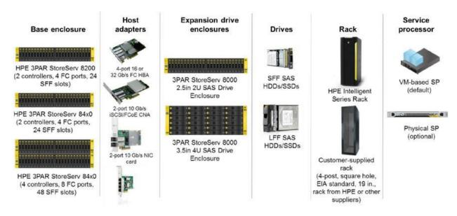
Figure 5-51 The basic building blocks of an HPE 3PAR StoreServ array
