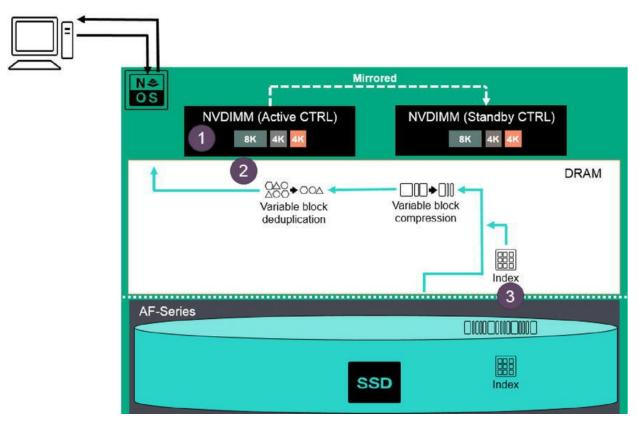
Figure 5-21 AF-Series read operation example
