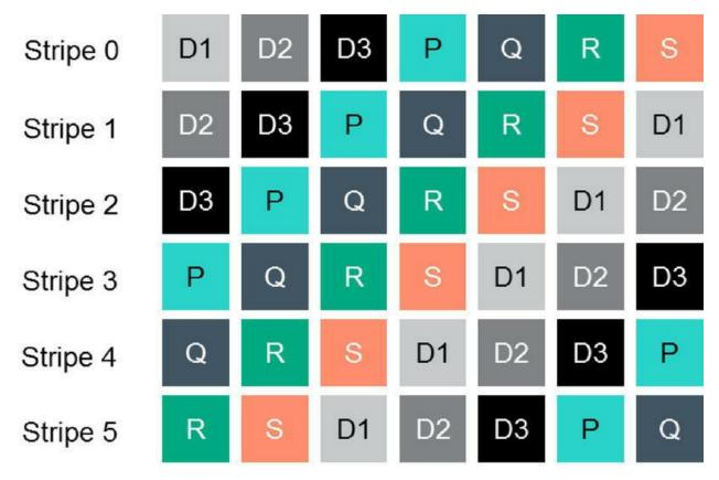
Figure 5-22 Triple+ parity layout
