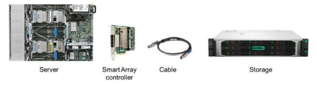
Figure 5-1 Components of Direct-attached storage
