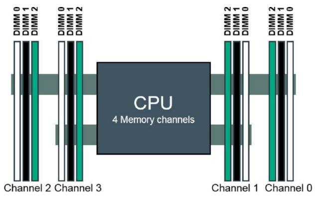
Figure 2-24 Gen9 with four memory channels per CPU
