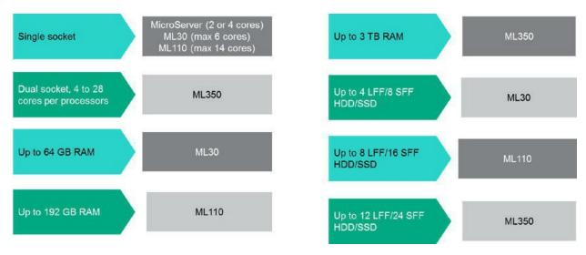
Figure 2-6 Selecting an HPE ML server platform, based on performance, memory, and storage requirements
