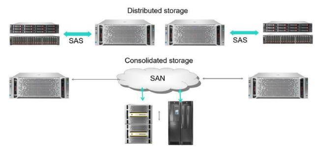
Figure 5-10 Comparing distributed to consolidated storage solution
