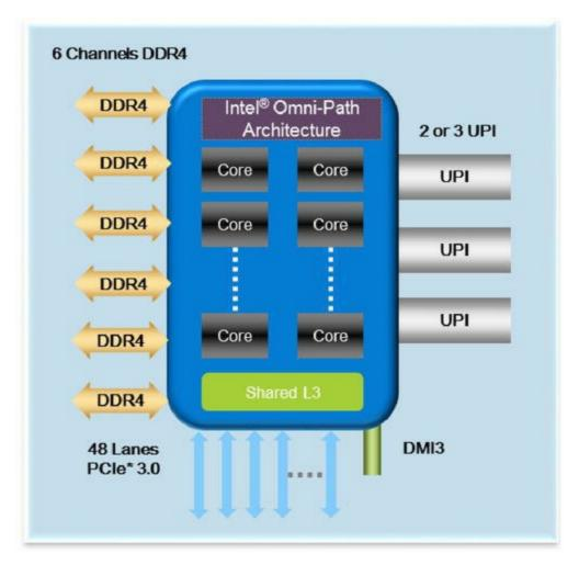
Figure 2-18 Intel<sup>®</sup> Xeon<sup>®</sup> Processor Scalable Family: Architecture
