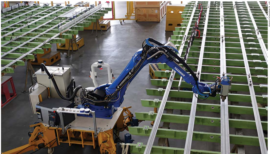
A drilling robot during a passenger-to-freighter conversion at ST Engineering.
