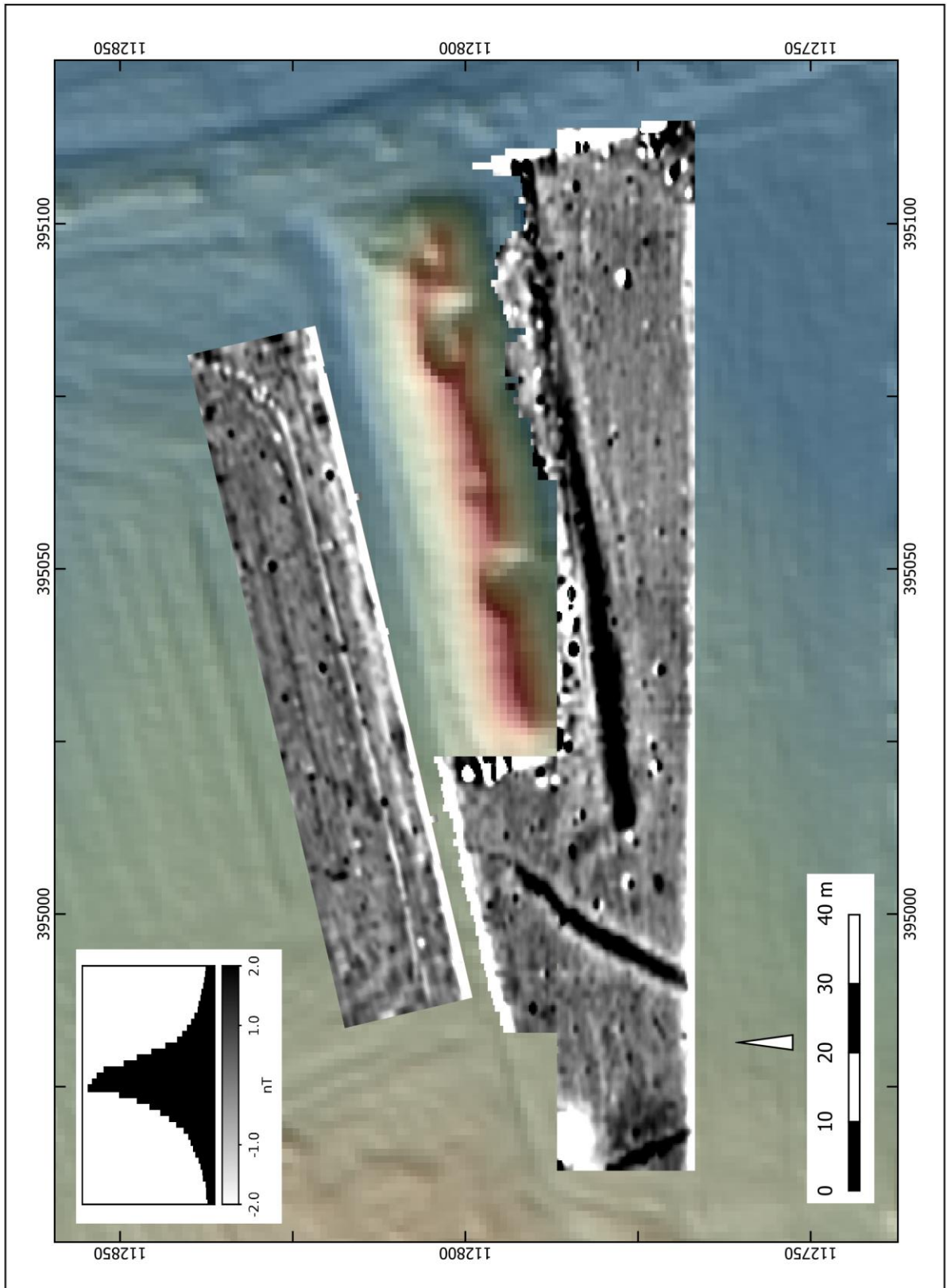
Figure 15: Chettle House Long Barrow: processed results: de-striped and interpolated. Linear greyscale, display range -2.0 to +2.0nT.
