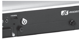
Swappable and lockable SATA3 HDD/SSD, Audio jack, USB 3.0 and CFast™
