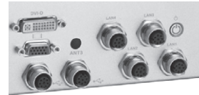
M12 type for Gigabit LAN, USB 2.0 & audio port
