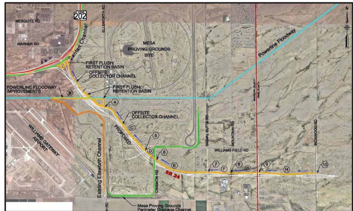
Figure 6 – Baseline SR 24 Off-site Drainage Improvements for the Ultimate Project (From ADOT, 2011, Figure 25, Modified)
