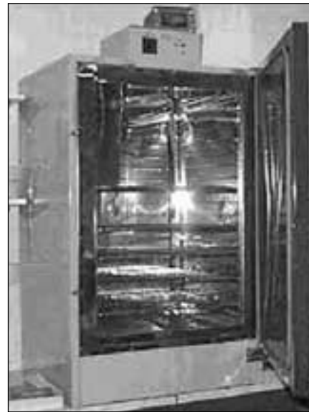
Figure 1: Example of a temperature controlled oven for drying sections
