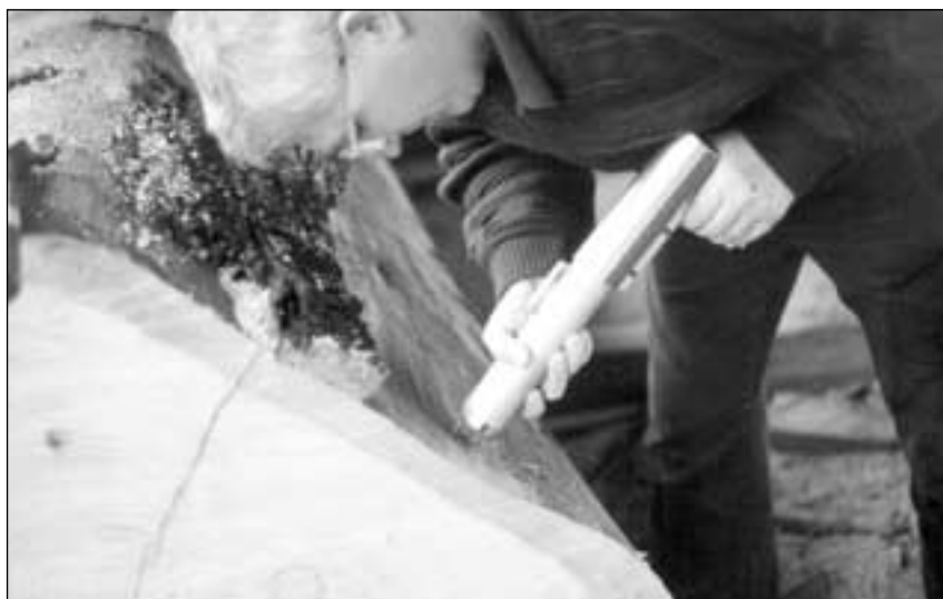
Figure 3. Pilodyn tester used for estimating basic density in a eucalypt log
