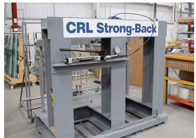
CRL Balustrade Test Rig
