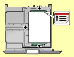
Insert the appropriate paper size card in the slot to indicate the size of the paper inside.
