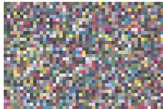
IT8.7/4 random layout (See the tutorial in Section 2.5.5 for visual clues on how to better recognize this layout.)
