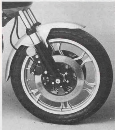
A 100/90 H 18 Metzeler surrounds an alloy wheel, cast iron rotors, 5.6-inch-travel fork and Brembo calipers.
