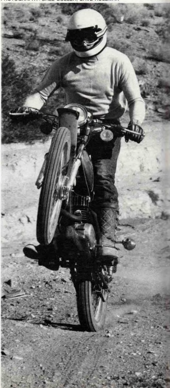
Front end steers well even with a trials tire. Tough plastic fender defies rocks, bends and weather.
