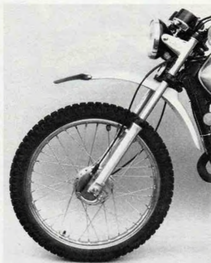
Front end steers well even with a trials tire. Tough plastic fender defies rocks, bends and weather.
