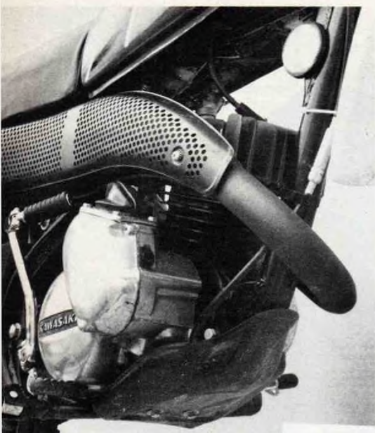
Despite a complete Mikuni carburetor behind that bulge, the engine only measures 11 inches wide.
