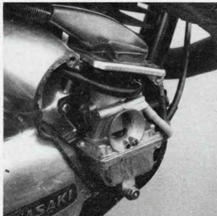
The side mounted Mikuni has an external main jet replacement cap-bolt in the float bowl.
