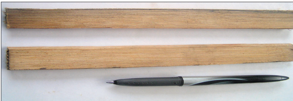
Figure 1: Pictorial representation of split-bamboo samples for testing tensile strength properties
