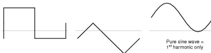
These waveforms are composed exclusively of odd harmonics.
