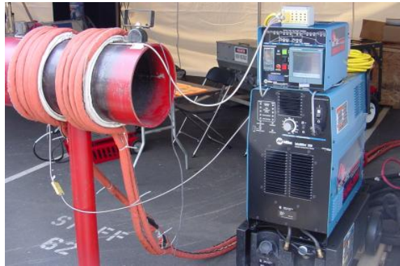
Induction heating: Primary insulated winding induces current into lossy iron pipe (secondary).
