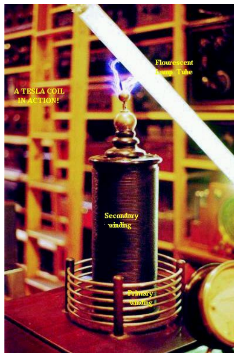
High voltage high frequency discharge from Tesla coil.
