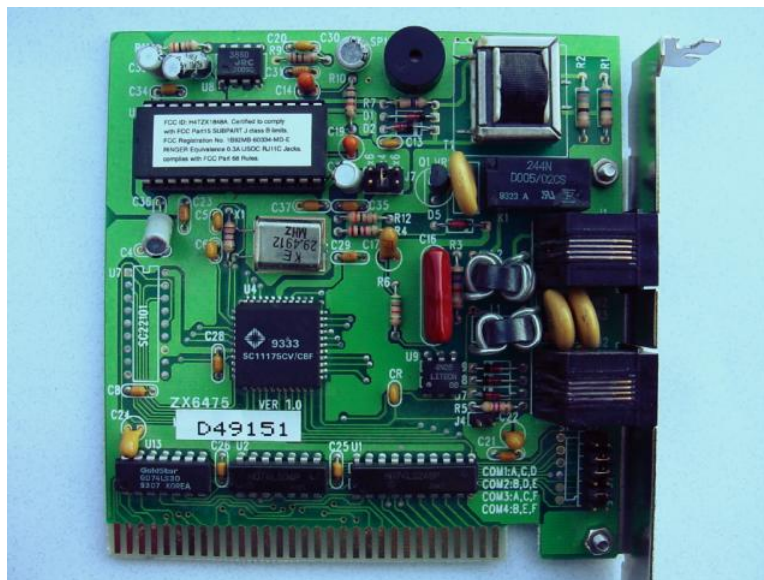
Printed circuit board mounted audio impedance matching transformer, top right.
