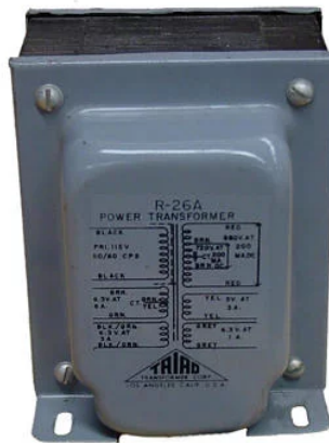
Photograph of multiple-winding transformer with six windings, a primary and five secondaries.
