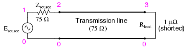
Shorted transmission line.
