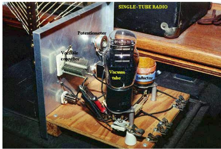
Variable capacitor tunes radio receiver tank circuit to select one out of many broadcast stations.
