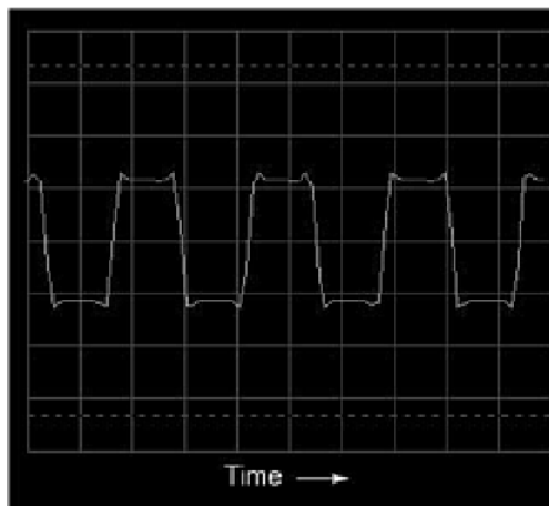
Oscilloscope time-domain display of a square wave
