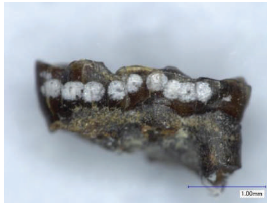
FIGURE 8.4 Laser ablation pits on a fossilised rodent tooth of Pliocene age (~3 million years old).
