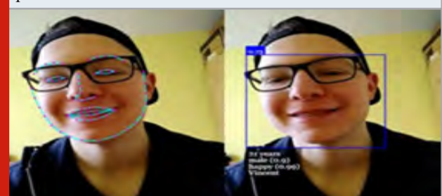
Figure 3: Input and output image showing a bounded box around the person and the recognized name of the person.
