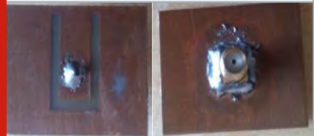
Figure 16: Fabricated U-shaped Patch Antenna: Front; Back View
