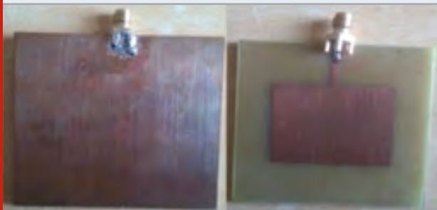
Figure 4: Fabricated Rectangular Patch Antenna: Front; Back View
