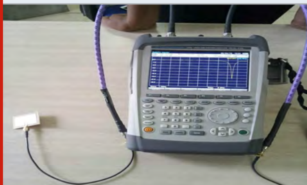
Figure 6: Measurement setup of antenna with VNA
