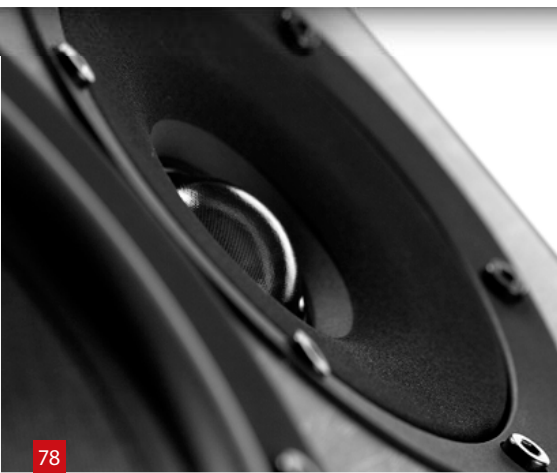
The WaveGuide result in a uniform treble dispersion pattern from 10kHz all the way down to the critical x-over point at 2kHz and thus secures a seamless transition to the mid/woofer – both when listening on and off axis.
