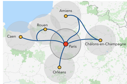
Fig. 11: Increased satellite-connectivity for Paris, by leveraging GTs located in nearby cities over high-bandwidth fiber.
