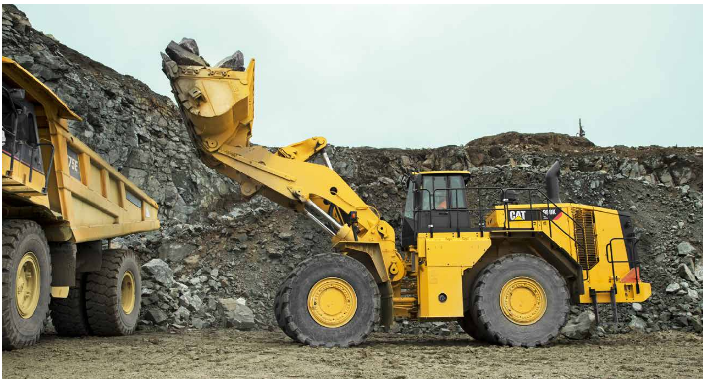
→ The 988K XE wheel loader is one of the largest construction machines in Sweden driven by a diesel hybrid.
