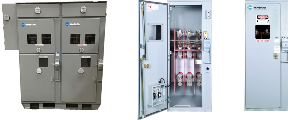
400A / 5kv "Mini" - Dimensions : 64"H x 25"W x 27"DDIN, E or R Fuse style – Max. 200E / 24R50ka w/ fuses / 14ka w/o fuses
