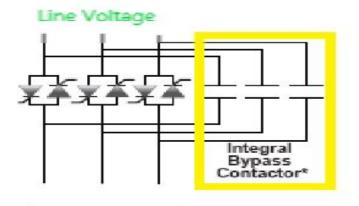
Fig 4. Typical – Basic Soft Starter configuration
