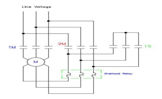
Fig 2. Basic Wye – Delta starter configuration
