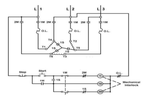
Fig 2. Typical – Open transition type Wye – Delta Starter
