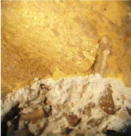
Micro-photograph of a colonette flute with gilding on a yellow iron oxide ground. Magnification ×30 (photo: Benton Kidd).
