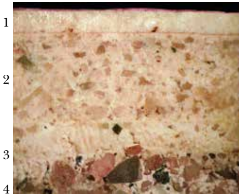
Micro-photograph of plastered fragment showing four layers of deposition. Layer 4: coarse aggregate base layer; Layer 3: intermediate layer; Layer 2: intermediate layer; Layer 1: fine layer of marble plaster with crystals burnished by saw during cutting.
