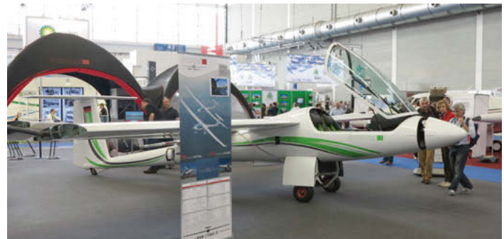
■ Stemme's S10 has had a facelift, shown for the first time at AERO 2013. Changes include a new look, a modified rim and braking system and new avionics (including engine monitoring system and the new Butterfly Vario). www.stemme.de
