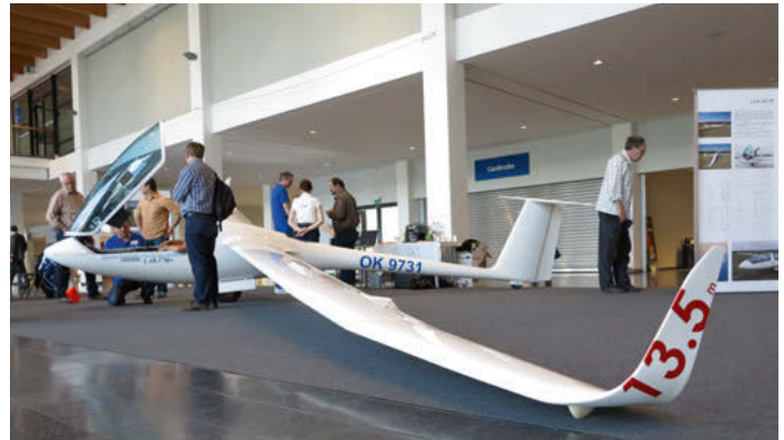
■ Sportine Aviacija displayed its LAK 17b fes . A LAK 17 MINI 13.5m sailplane is now available in four versions: pure, self-launching, FES and Acro FES. www.balticsailplanes.co.uk
