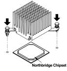
Insert the push pins into the mounting holes on the motherboard and ensure they remain firmly in place.
