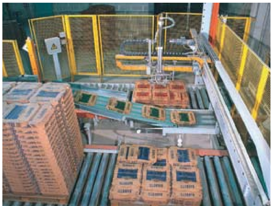
Automatic empty bag de-palletizer supplied for Cementerie Aldo Barbetti in Italy.
