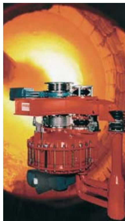
Pfister produces rotary weigh feeders for coal firing of cement kilns.
