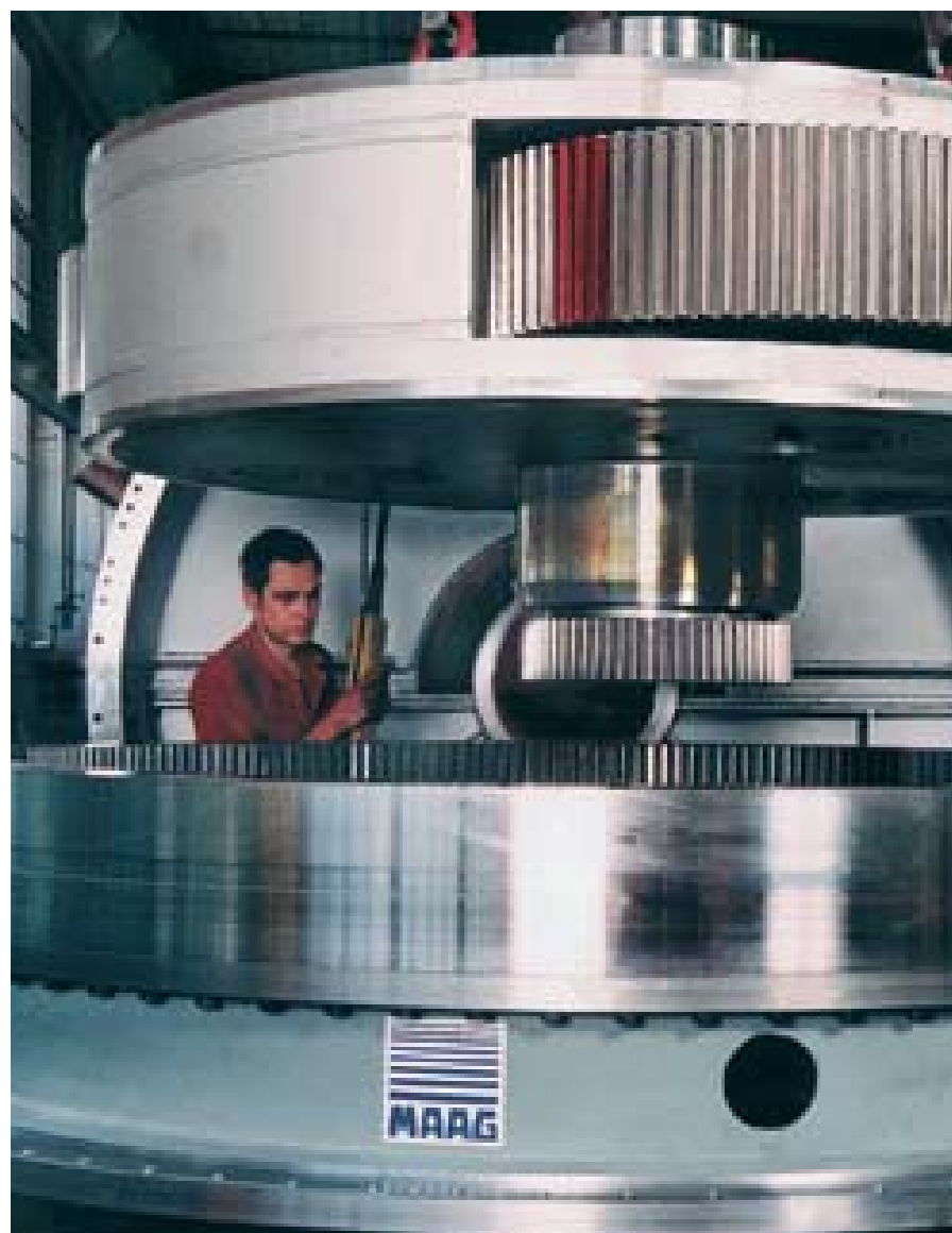
Planetary gear being assembled at MAAG Gear in Switzerland.
