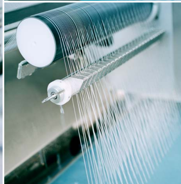
One of Gambro's largest production facilities for synthetic dialysis membranes and dialyzers is located in Hechingen, Germany. The membrane of the Polyflux dialyzer, which is being produced here, consists of a unique polymer blending. In a sophisticated but well controlled process a polymer solution is being transformed into a hollow-fiber. Depending on the type a Polyflux dialyzer contains between 8,000 – 12,000 of these fibers. Jakob Schmidt controls that the process runs smoothly and ensures that all fibers are being separated and that not one single fiber snaps.
