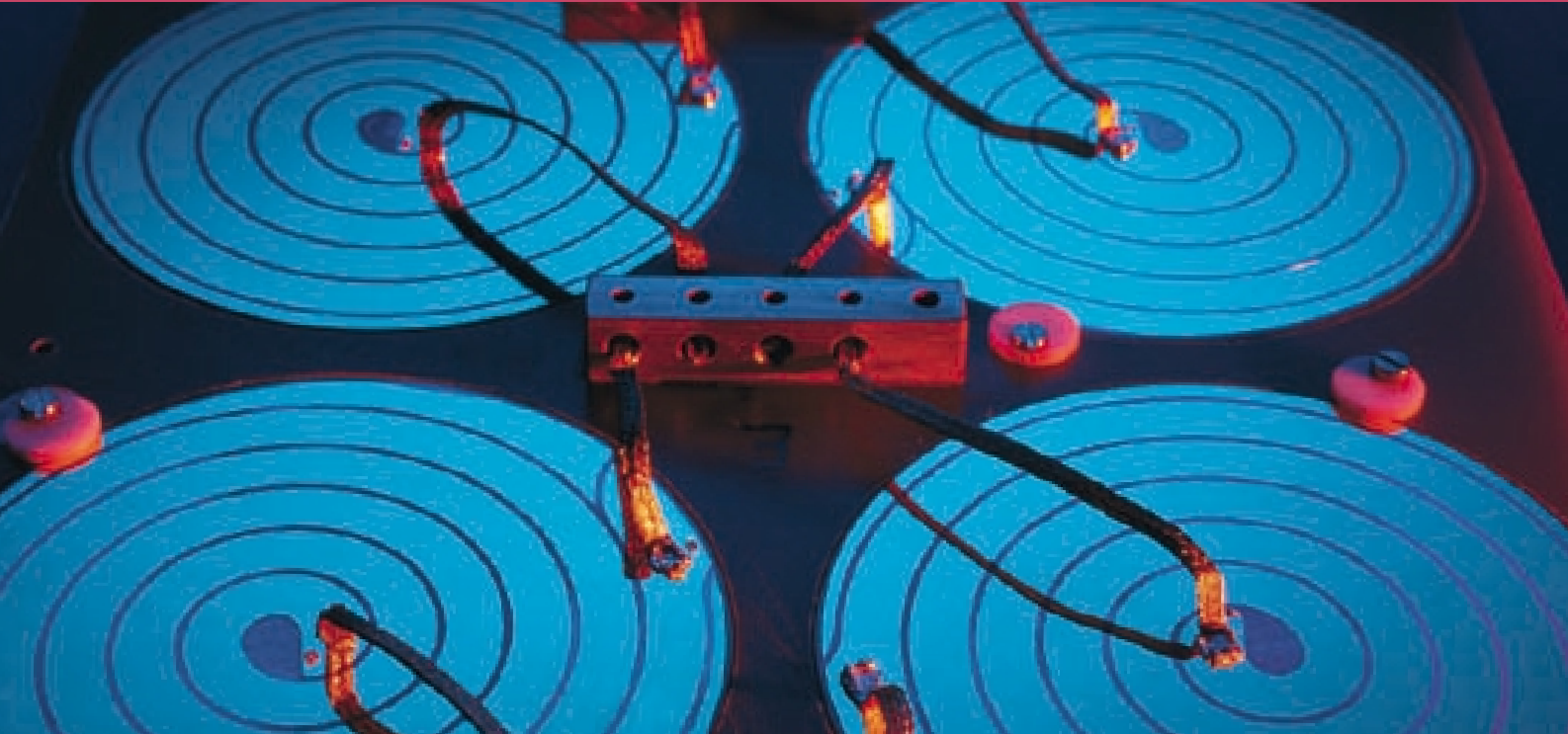
Superconducting current limiters function as resettable fuses in the event of a short circuit, promising major cost advantages.
