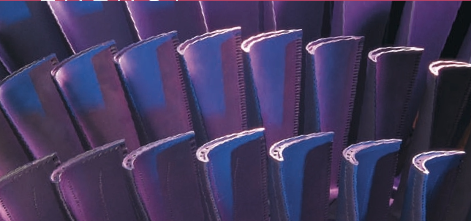
A ceramic coating improves the durability and efficiency of gas turbine blades.
