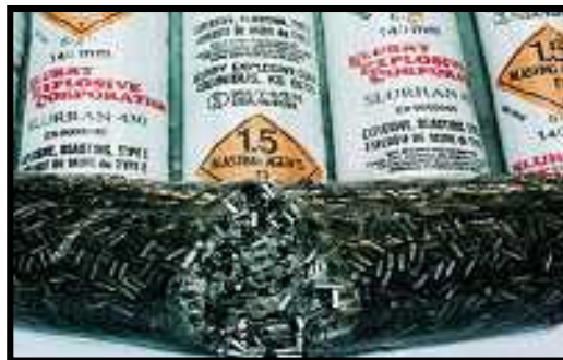
Figura 2-32 SLURRIES. Fuente: Slurry Explosive Corporation.
